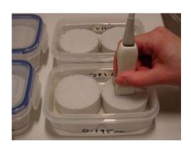
Figure 2: Image of the modified Edinburgh Pipe Phantom to assess preclinical ultrasound scanners
